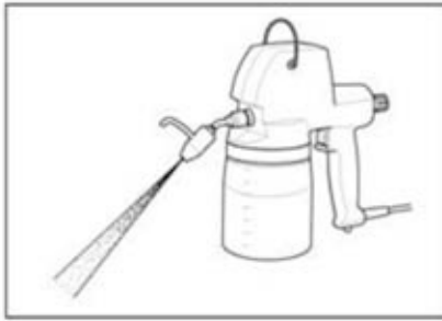
Nozzle handle upwards. Flushing with sharp jet.
