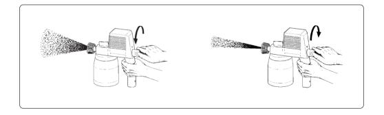
• Have you been spraying liquid with particles? If so, some of these may have got into the chamber and stoped the piston from moving properly. Please take the piston out of the pump unit and follow the next step.
