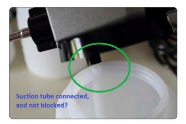
• You are struggling to fit the suction tube extension cup: Pull out the end of the suction tube and fit the metal adapter piece first. Then pull the cup up and screw it into the pump housing - the thread is on the outside of the cup.
