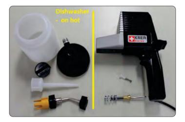
Please separate the electrics and washing all in the dishwasher at 150F+ (except the ball (6) and atomiser insert (7)) - then reassemble and try spraying. This is particularly important if you have i) been spraying particles or ii) left high viscosity materials dry.
